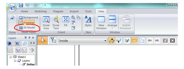
Once you have drawn something in the 2D Model view, switch to your Sheet and place your drawing at required scale using Sketching > Create Drawing from 2D Model as follows:
