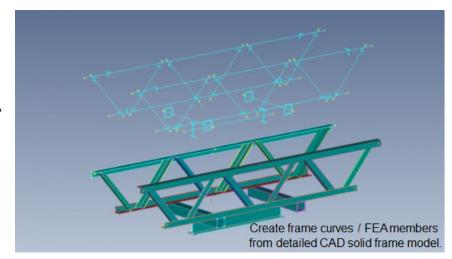
properties assigned - from CAD solid model of frame/truss members.
