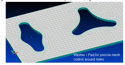
Geometry Copy / Rotate / Reflect can simultaneously replicate mesh (incl regions, BCs, loads and coords used for these). Plus, more options to specify orientations of transformed entities. Also allows optional control of relative numbering of new entities.
