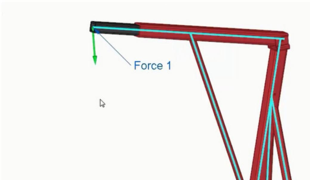
Once the study is set up, running a beam analysis is fast and efficient, as Solid Edge Simulation doesn't need to worry about the exact frame geometry to solve for the reaction forces on its members.
