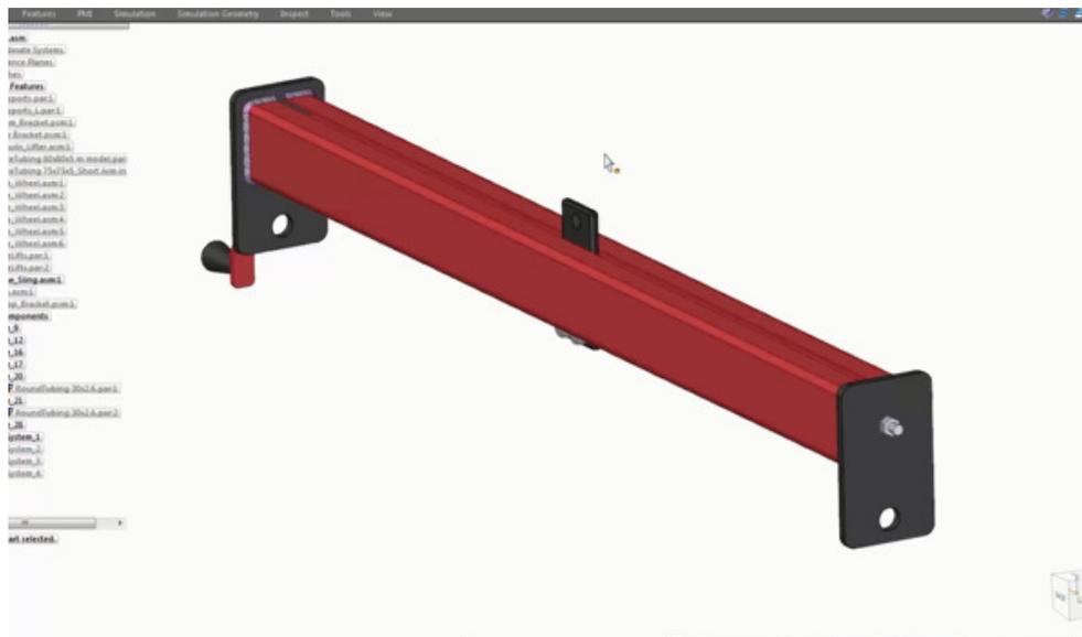
Imagine that you have a requirement that the bolt can't bend more than 1mm, because the adjustment bracket wouldn't work properly.
