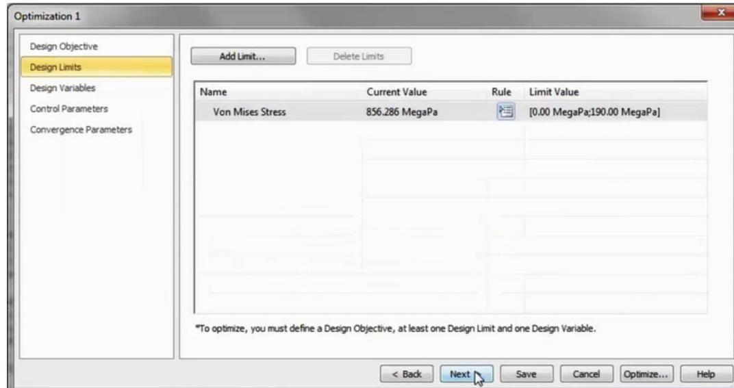
Next, define limits of the parts, such as stresses that they cannot exceed, and define what changes you want Solid Edge to make, such as thicknesses and lengths of components.
