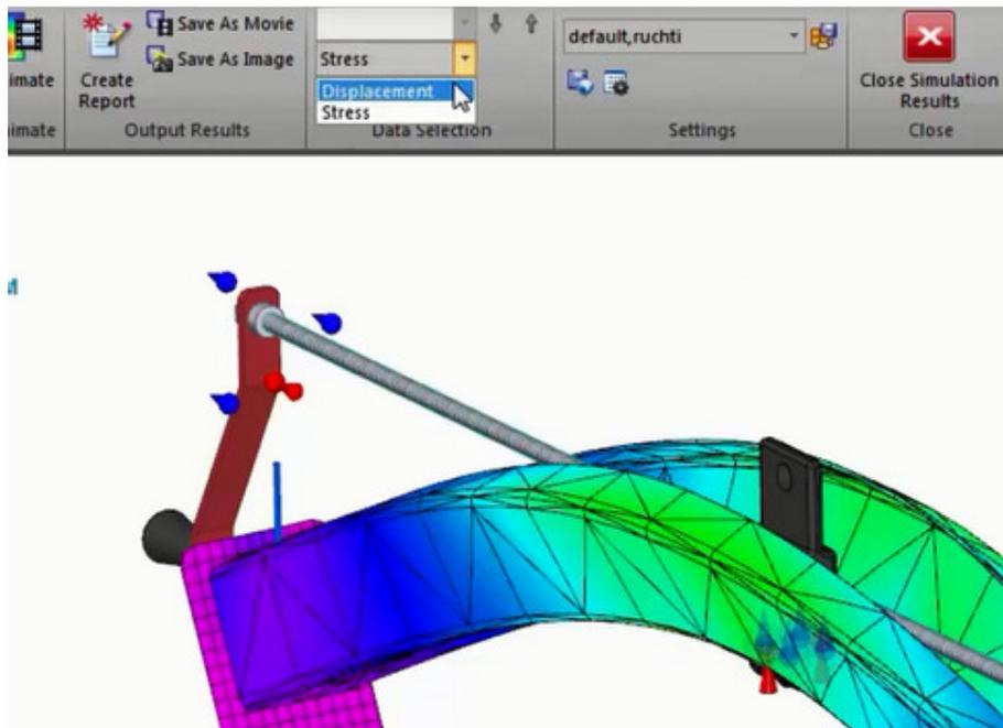
If you don't get your desired results the first time—such as, if our beam from the previous example has a displacement of more than 1mm—Solid Edge synchronous technology allows for easy changes to your design depending on your end goals. However, rather than manually making time-consuming changes to try to dial in the appropriate results, Solid Edge provides a great tool to automate and optimize your design – Simulation Optimization.
