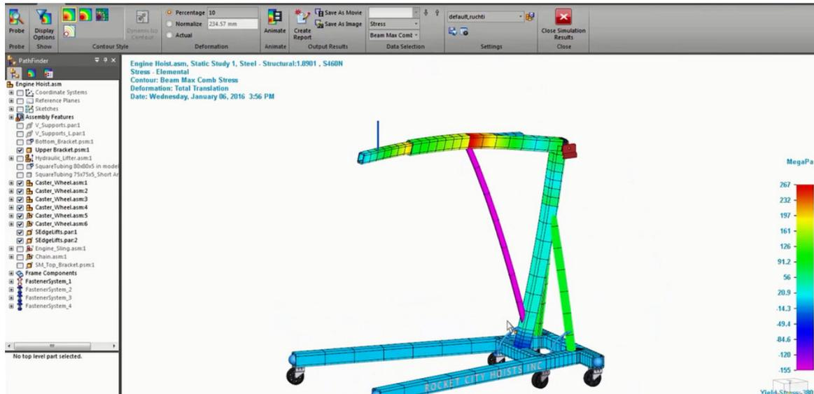
Once solved, Solid Edge provides an easy to understand readout of the results. If changes need to be made, Solid Edge allows you to edit the model quickly and easily, and then simply rerun the existing simulation study to review results of the change.
