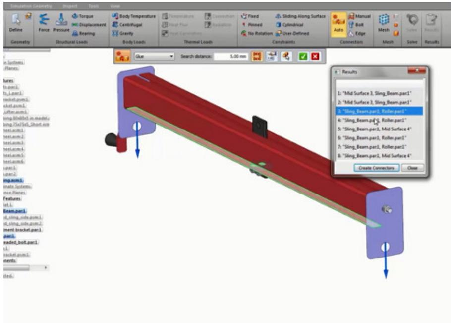
Once everything is set up, you can mesh and solve the study. Solid Edge gives users complete control over the mesh settings for both solid and surface meshes. You can easily change your view of results, for example, from stress distribution to displacement, using a dropdown.
