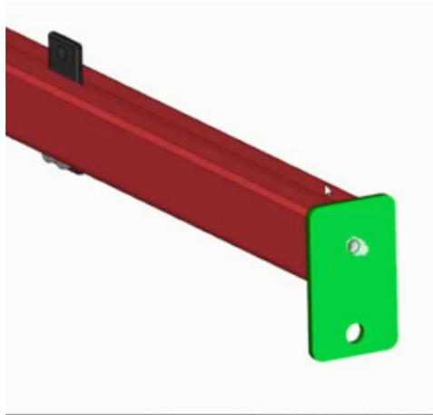
With the end caps defined, you can then set up the study. No matter the type of study being run, common steps are used to set them up. You have geometry, loads, and constraints—just like in beam analysis—but in the assembly study you need to define how the parts connect together (this was done automatically in the beam analysis based on the proximity of the beams to one another).
